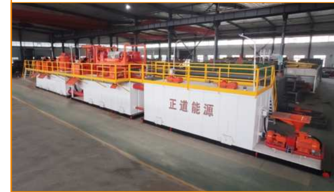
02 煤层气钻井固控系统 CBM Drilling Rig Mud System
