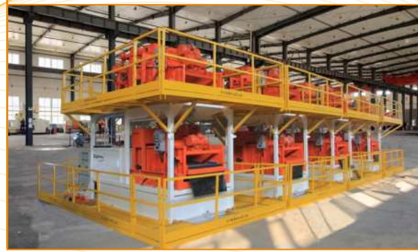
04 盾构/顶管泥水分离系统 TBM Separation Plant
