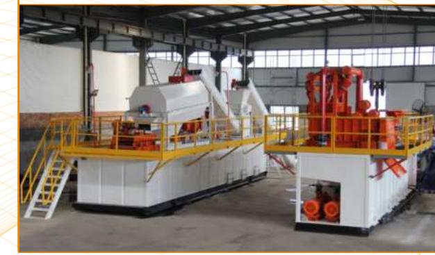
07 含油污泥处理系统 Oil Sludge Treatment Plant
