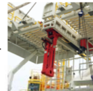
Mechanical arm on RB • Hydraulically driven folding arm • Small size, light weight • 2 7/8 - 9" Wide range of pipe holding
