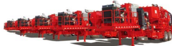
SGJ600-30T Trailer-mounted cementing unit
