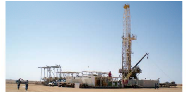
SZJ180T(ZJ30DBT) Trailer-mounted drilling rig working in Oman
