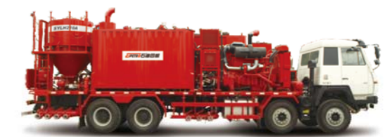
Fracturing fluid continuous mixing truck
