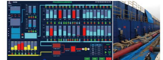
Control interface for automatic liquid supply
