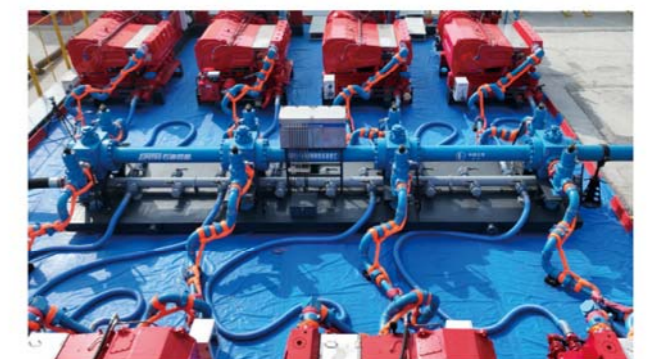
140MPa Large-size Remote-Controlled Fracturing Manifold Device
