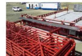
Onsite application of hydraulic pipe box (Pipe out)
