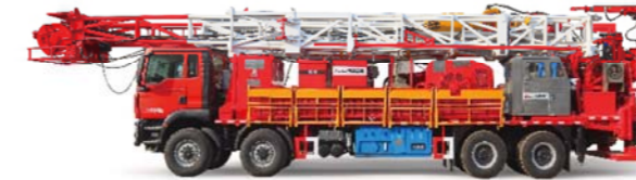
SXJ350D(XJ900) workover rig (Electric drive)
