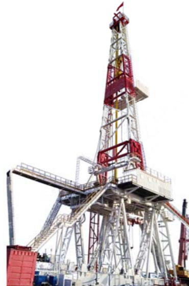
Substructure for 9000m Double-lifting drilling rig
