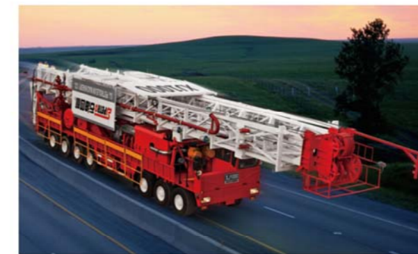
SXJ1000(XJ2250) workover rig (Diesel engine drive)
