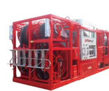
Power control skid
