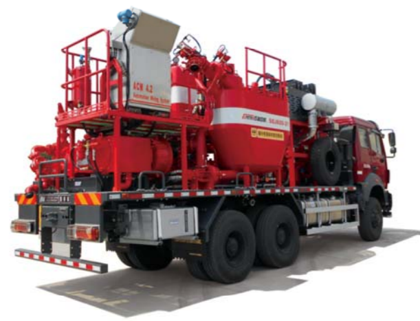
SGJ600-21 Single pump intelligent cementing truck
