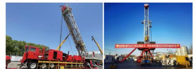
3000m Super single automated rig raising-up mast
