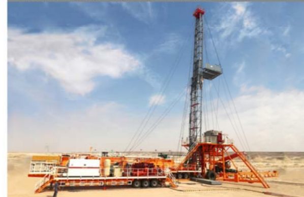
SZJ180CZ(JZ30) Truck-mounted drilling rig (8 axles)
