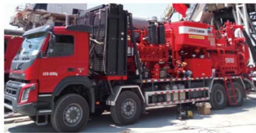
SGJ2500-38 High power cementing truck working in Weiyuan, Sichuan.
