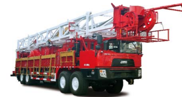
SXJ450(XJ1100) workover rig (Diesel engine drive)
