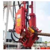
Hydraulic elevator • The anti-freezing design of hydraulic elevator can prevent its failure caused by the frozen liquid from the pipe string.
