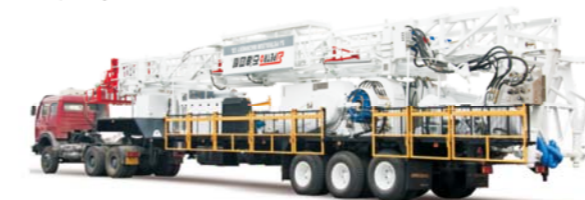
XJ450T Trailer-mounted workover rig (Diesel Engine Drive)
