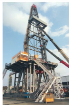
8000m continuous-lifting drilling rig
