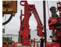
Lift-hold rig floor manipulator
