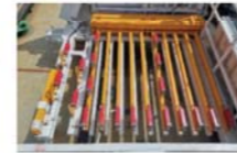
Power racking board • Automatically adjustable fingers. • Satisfying the arrangement of different pipe strings.
