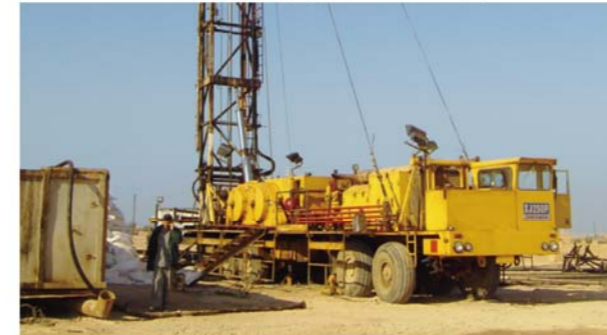
XJ250P flushing & workover rig working in Syria
